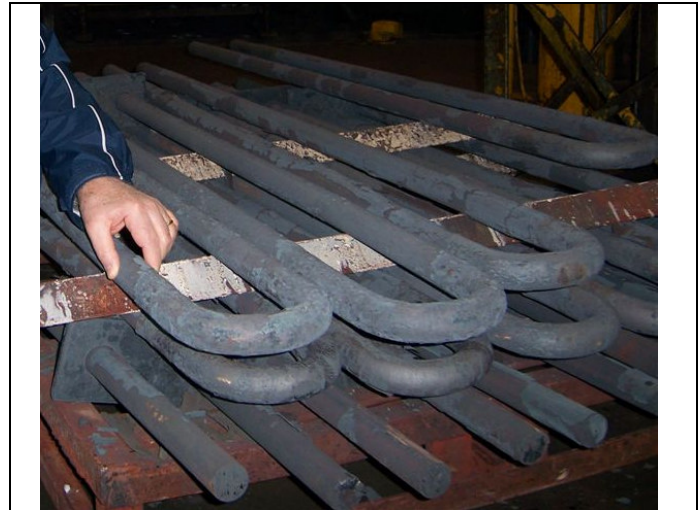
Part way through production - large, extra heavy duty strengthened steel U-Bolts custom ordered for bridge construction.
